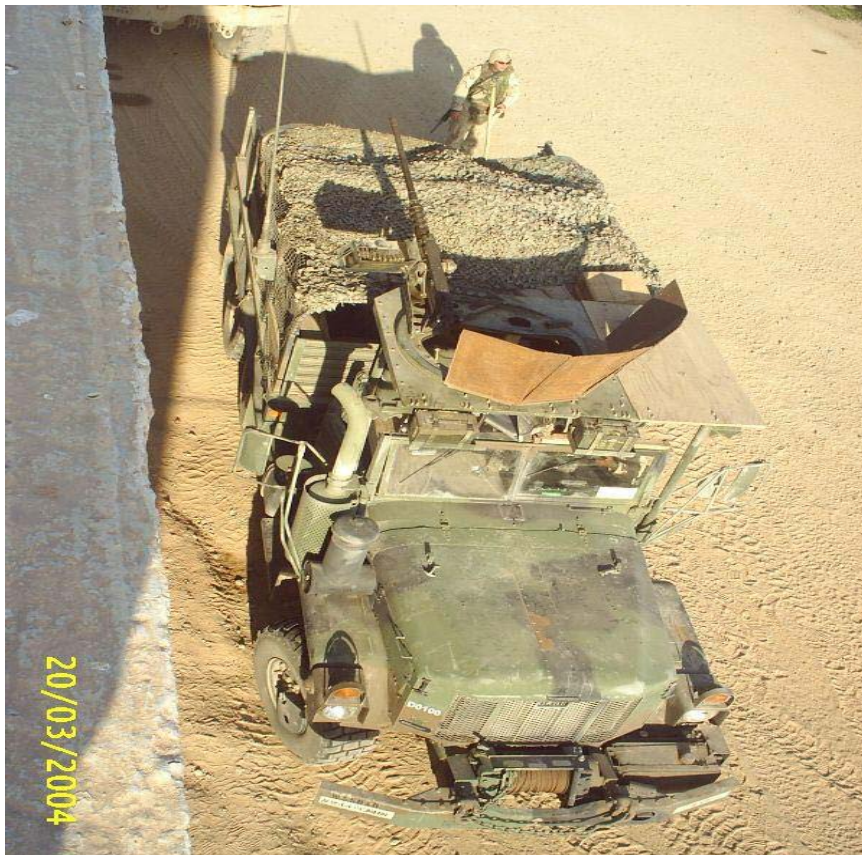
Figure 6.6 Gunner's shield and camouflage for the bed of the truck. MODIFIED FROM CALL HANDBOOK, SOSO NO 3-20.
